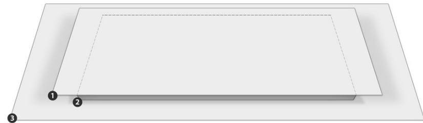
1. Top Metal Print | 2. Gatorfoam Float Mount | 3. Bottom Metal Print
